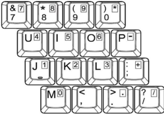
Figure 11. 15-key Numeric Keypad
