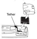
Replace the battery cover, pressing down firmly while securing the latches.
