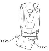
2. Insert the lithium-ion battery in the battery compartment with the battery tether positioned properly (as shown below), making sure the battery snaps into place.
