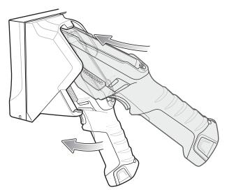
Figure 2-12 Insert TC8000 into Cradle
