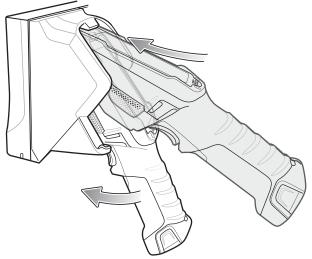
Figure 2-3 Insert TC8000 into Cradle
