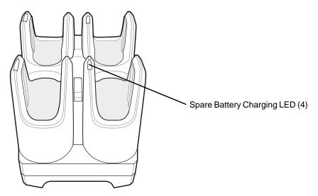
Figure 2-19 4-Slot Battery Charger
