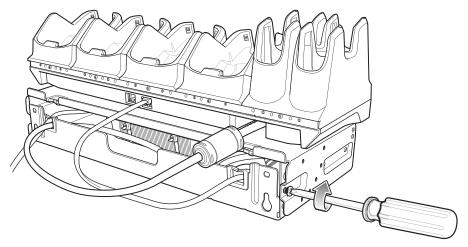
Figure 2-38 Secure Top and Bottom Tray
