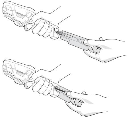
Figure 1-8 Battery Installation
