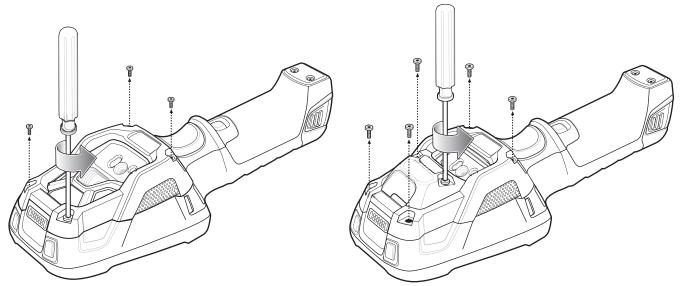
Figure 1-3 Remove Screws
