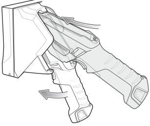
Figure 2-6 Insert TC8000 into Cradle
