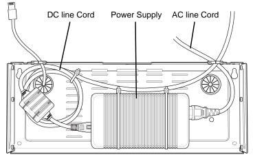
Figure 2-32 Power Supply in Bottom Tray
