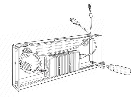
Figure 2-51 Horizontal Installation - Tighten Screws
