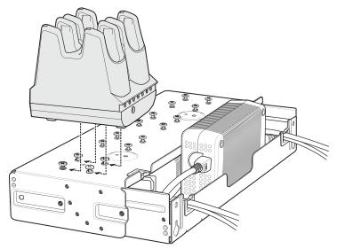
Figure 2-42 Align Chargers on Studs
