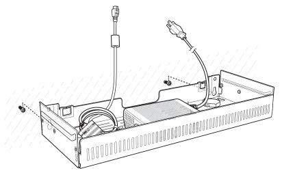
Figure 2-53 Horizontal Installation
