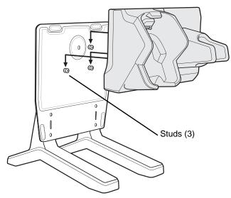
Figure 2-23 Install Cradle onto Desk Mount
