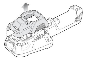
Figure 2-56 Lift Rear Bezel
