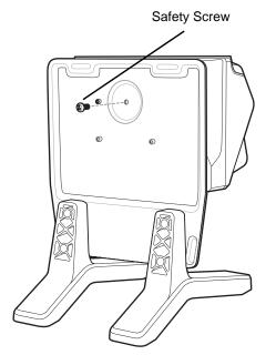
Figure 2-24 Install Safety Screw
