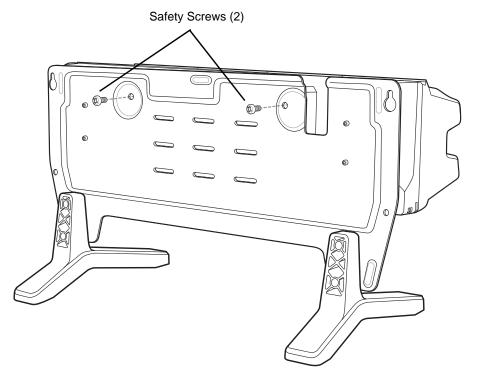
Figure 2-28 Install Safety Screws
