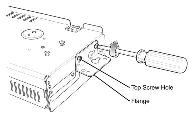
Figure 2-45 Flange Vertical Position (5-Slot Cradles)
