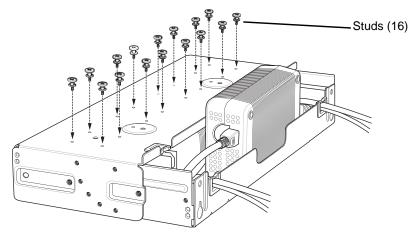
Figure 2-41 Install Studs
