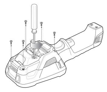
Figure 2-55 Remove Screws
