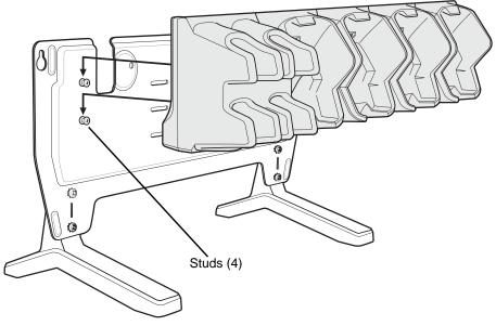
Figure 2-27 Install Cradle onto Desk Mount
