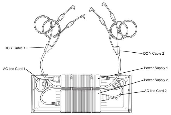
Figure 2-39 Power Supplies in Bottom Tray
