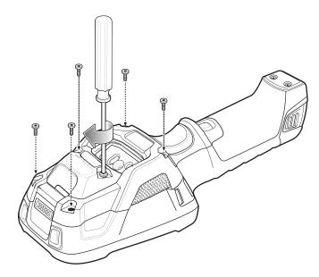
Figure 2-59 Secure Back Bezel
