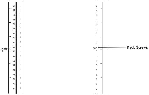
Figure 2-47 Install Rack System Screws
