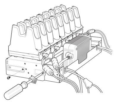
Figure 2-44 Secure Top Tray to Bottom Tray
