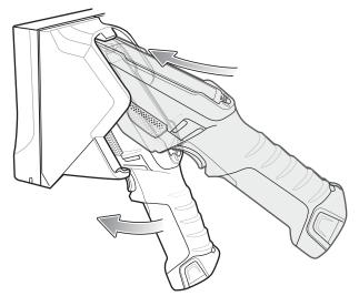
Figure 2-18 Insert TC8000 into Cradle
