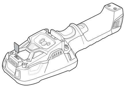
Figure 1-5 Insert microSD Card
