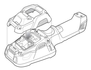
Figure 2-58 Align Back Bezel
