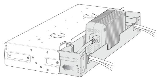
Figure 2-40 Slide top Tray onto Bottom Tray
