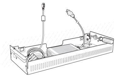
Figure 2-54 Horizontal Installation - Tighten Screws
